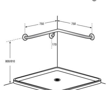
This product is AS1428.1 compliant (accessible compliant) when installed in accordance with the guidelines.
